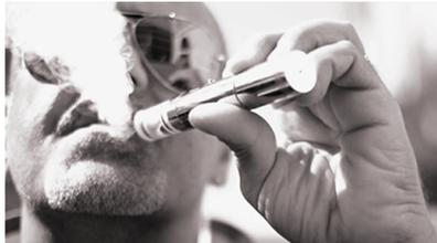
E-cigarettes come in two parts: in one end there is liquid nicotine, and in the other a rechargeable battery and an atomizer. When the user sucks, the liquid nicotine is vaporized and absorbed through the mouth.
